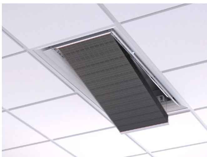
Figure 12. Removing the face plate and folding out the coil for accurate cleaning in the event of high hygiene requirements. Note! requires the product to be ordered with the accessory, fold-out coil, and that flexible connection hoses are used on the water side.
